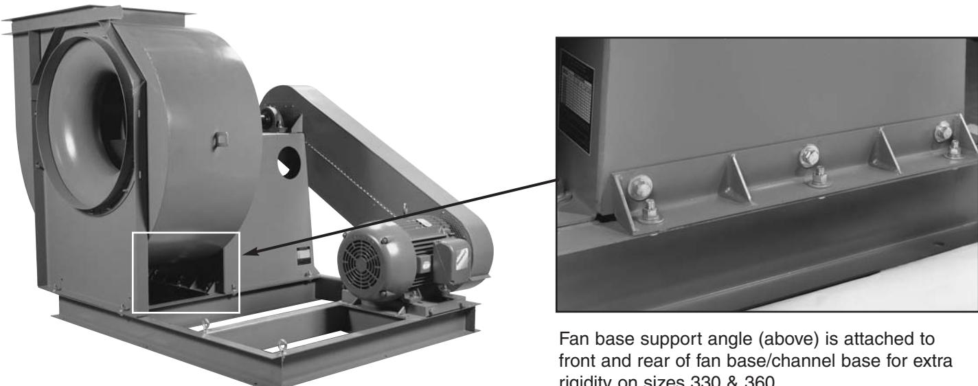
Fan base support angle (above) is attached to front and rear of fan base/channel base for extra rigidity on sizes 330 & 360.
